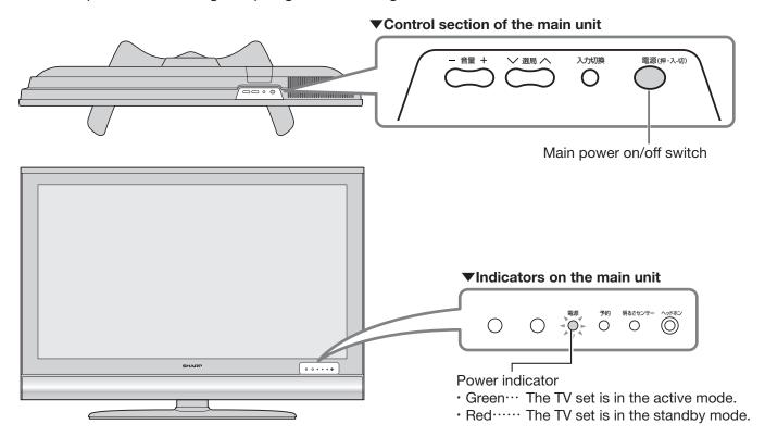
② After the main power is turned on, press the active/standby (電源) button on the remote control to engage the TV set in the active or standby mode.
