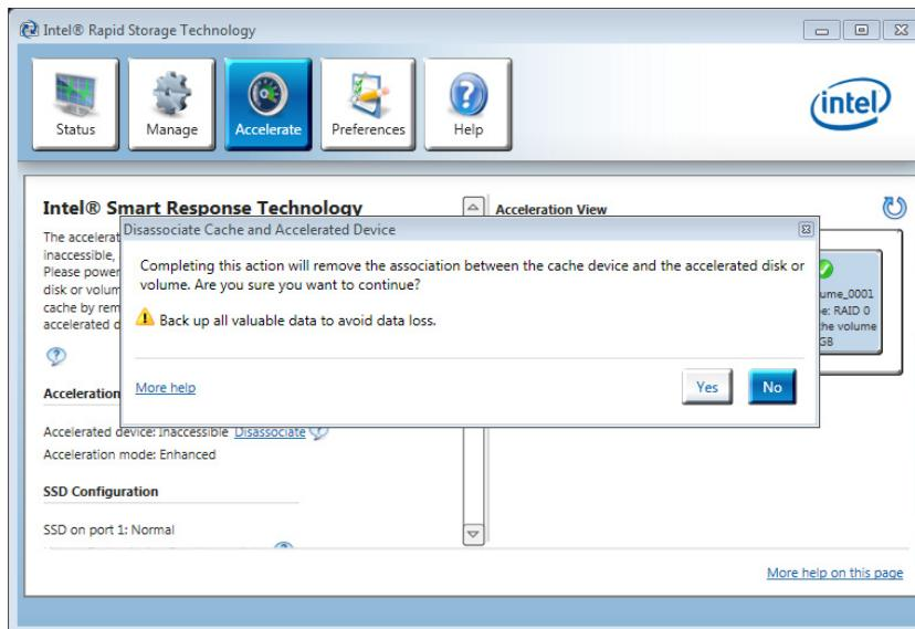
"Clicking Yes will return the mSATA or SSD cache device to a blank non-accelerated state, at which point it can be reconfigured by following the configuration steps described in the configuration section above.
