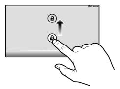
To turn off your device, press **a**, and tap **Shutdown > Power off > OK**. Alternatively, you can press and hold the Power button, and tap **Power off > OK**.
