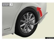
For vehicles with 15 inch wheels, remove the wheel ornament using the wrench.
