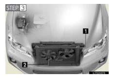
After the hybrid system has cooled down sufficiently, inspect the hoses and radiator core (radiator) for any leaks.
