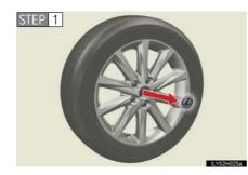
Vehicles with a 16 or 17 inch wheel: Before stowing the flat tire, remove the center wheel ornament by pushing from the reverse side.
