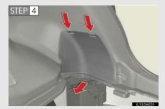
Remove the 12-volt battery maintenance cover.
