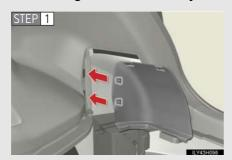
Insert the 2 tabs on the far side of the cover into the holes.
