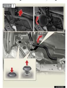
For the right side only: Remove the securing clips and unclip the engine coolant reservoir hose. Then lift up the air cleaner inlet duct.
