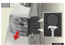
Open the back door and remove the covers and bolts, and remove the lamp assembly by pulling it directly backward from the rear of the vehicle.
