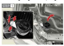
For the right side only: Move the washer fluid filler opening.
