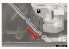
Non-flat dipstick: Reinsert the dipstick fully with its protruding areas ( in the illustration) pointing towards engine.
