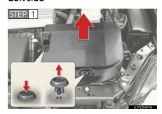
Remove the power control unit cover.
