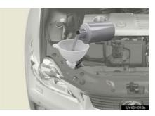
If any washer does not work or the warning message appears on the multi-information display, washer tank may be empty. Add washer fluid.
