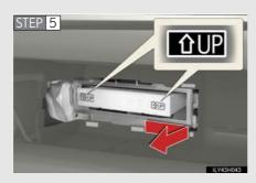
Slide and pull out the filter. Replace it with a new one.
