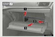
Open the glove box. Lift and remove the partition.
