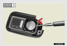
Remove the depleted battery.
