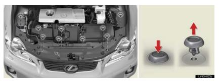
■ Installing the clips
