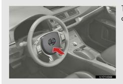
To sound the horn, press on or close to the or mark.
