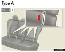
Latch the hooks of the lower straps onto the LATCH anchors. If the child restraint has a top tether strap, the top tether strap should be latched onto the top tether strap anchor. For owners in Canada:
