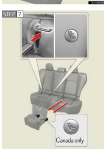
Latch the buckles onto the LATCH anchors. If the child restraint has a top tether strap, the top tether strap should be latched onto the top tether strap anchor.
