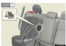
Open the anchor bracket cover, latch the hook onto the anchor bracket and tighten the top tether
