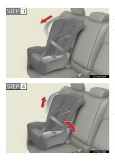
Fully extend the shoulder belt and then allow it to retract slightly in order to activate the ALR lock mode.
