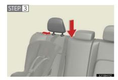
Outside only: Adjust the head restraint to the downmost position.
