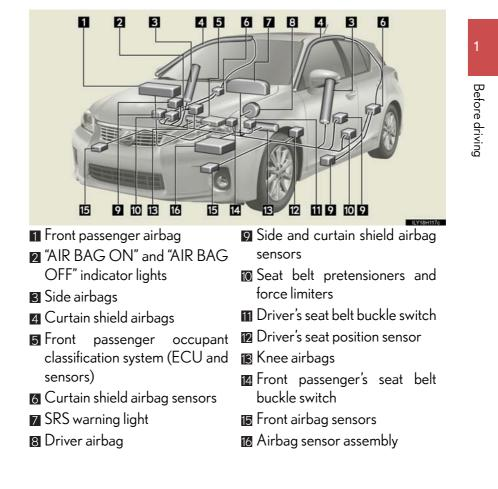
Your vehicle is equipped with ADVANCED AIRBAGS designed based on the US motor vehicle safety standards (FMVSS208). The airbag sensor assembly (ECU) controls airbag deployment based on information obtained from the sensors etc. shown in the system components diagram above. This information includes crash severity and occupant information. As the airbags deploy, a chemical reaction in the inflators quickly fills the airbags with non-toxic gas to help restrain the motion of the occupants.
