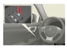
Press the switch down to lock the passenger window.
