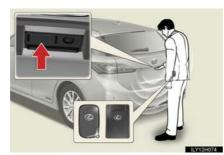
Press the back door opener switch to unlock all the doors.
