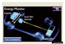
The flow of energy is displayed on the navigation system screen.
