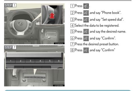
E Pressing this switch turns the voice command system on. Say a command after the beep.
