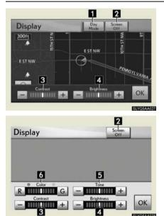
Press the "DISP" button on the Remote Touch to show the "Display" screen.
