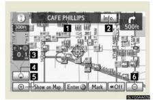
To scroll over the map, place the pointer in a position near the desired destination and then press and hold the "ENTER" button on the Remote Touch.
