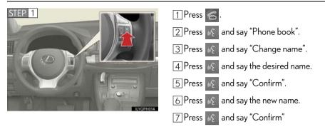
: Pressing this switch turns the voice command system on. Say a command after the beep.
