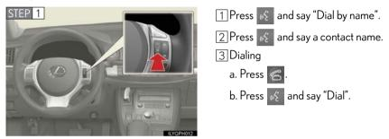
See Pressing this switch turns the voice command system on. Say a command after the beep.
