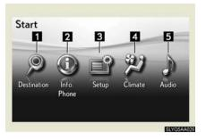
Press the "MENU" button on the Remote Touch to display the "Start" screen.
