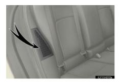
There is an air intake vent on the side of the rear right seatback for the purpose of cooling the hybrid battery (traction battery). If the vent become blocked, the hybrid battery may overheat, leading to a reduction in hybrid battery output.
