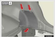
Remove the 12-volt battery maintenance cover.
