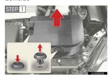
Remove the power control unit cover.
