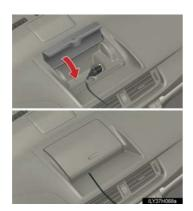
The gap in the lid allows power cables to be passed through even when the lid is closed.
