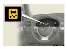
If the vehicle is in danger of slipping or if any of the drive wheels spins, the slip indicator light flashes to indicate that the VSC/TRAC systems are operating.
