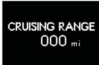
Displays the estimated maximum distance that can be driven with the quantity of fuel remaining.
