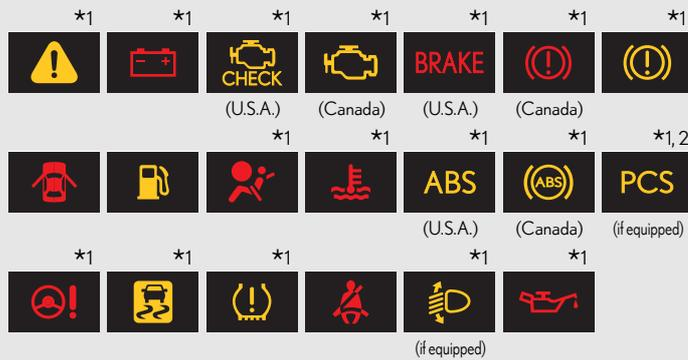
\*1: These lights turn on when the "POWER" switch is turned to ON mode to indicate that a system check is being performed. They will turn off after the hybrid system is on, or after a few seconds. There may be a malfunction in a system if a light does not come on, or if the lights do not turn off. Have the vehicle inspected by your Lexus dealer.
