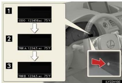
Switches between odometer and trip meter displays. When the trip meter is displayed, pressing and holding the button will reset the trip meter.
