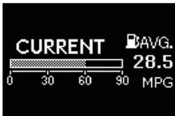
Displays the instant fuel consumption and average fuel consumption after refueling.
