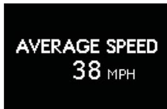
Displays the average vehicle speed since the function was reset
