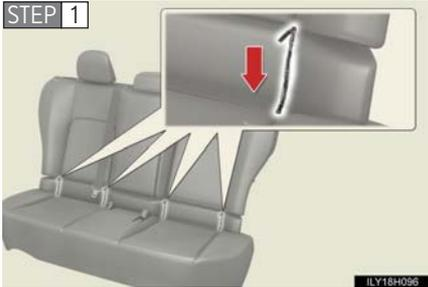
Open the fasteners on the lower part of the seatback.
