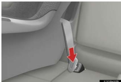
Press the buckle release button and fully retract the seat belt.
