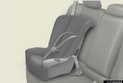
Seat belts equipped with a child restraint locking mechanism (ALR/ELR belts except driver's seat belt) (→P. 90)
