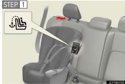
Secure the child restraint system using the seat belt or the LATCH anchors, press the lock release button, and raise the head restraint.
