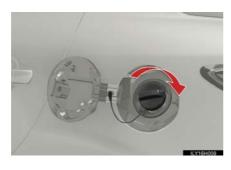
After refueling, turn the fuel tank cap until you hear a click. Once the cap is released, it will turn slightly in the opposite direction.
