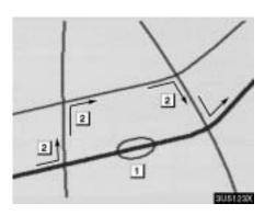
This picture shows an example of how the system would guide around a delay caused by a traffic jam.
