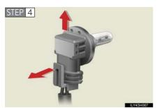
Unplug the connector while pulling the lock release.
