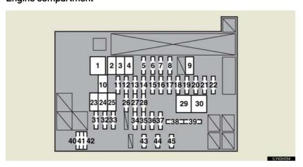
Fuse Ampere Circuit DC/DC 125 A Inverter and converter 1 50 A 2 HTR Air conditioning system **RDI** 30 A 3 Electric cooling fans **CDS** 30 A Electric cooling fans 4 5 RAD NO.1 15 A Audio system, navigation system S-HORN 10 A Alarm, navigation system 6 **ENG W/P** 30 A Cooling system 7 7.5 A ABS MAIN NO.2 Electronically controlled brake system 8 H-LP CLN 30 A 9 Headlight cleaner P CON MTR 30 A P position control system
