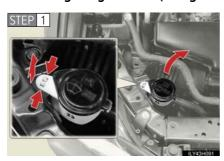
For the right side only: Move the washer fluid filler opening.
