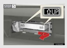
Slide and pull out the filter. Replace it with a new one.
