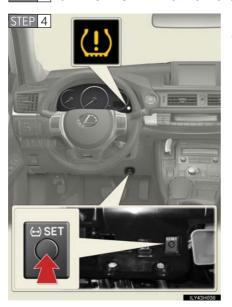
Press and hold the tire pressure warning reset button until the tire pressure warning light flashes slowly 3 times.
