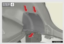
Remove the 12-volt battery maintenance cover.
