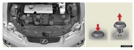
n Installing the clips
