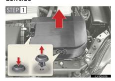
Remove the power control unit cover.
