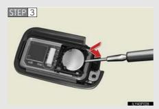
Remove the depleted battery.
