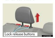
Pull the head restraint up while pressing the lock release buttons.
