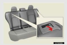
Pull up the seatback lock release lever until the lock is released.
