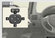
To adjust the mirror, press the switch.
