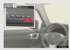
While pressing the "SET" button, or within 3 seconds after the "SET" button is pressed, press button 1, 2 or 3 until the signal beeps.
