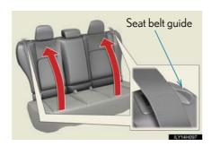
To avoid trapping the seat belt between the seat and the inside of the vehicle, pass the seat belt inside the seat belt guide and then return the seatback securely to the locked position.
