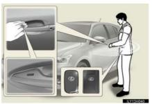
Touch the lock sensor (the indentation on the upper part of the door handle) to lock the doors.
