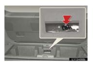
Lift the center deck board and then push down the lever in the hole.
