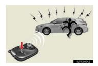
When (() is pressed for longer than about one second, an alarm will sound intermittently and the vehicle lights will flash to deter any person from trying to break into or damage your vehicle.
