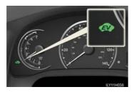
The EV indicator comes on when driving the vehicle using only the electric motor (traction motor).
