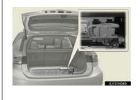
1 Never try to open the service plug access hole located in the luggage compartment. The service plug is used only when the vehicle is serviced and is subject to high voltage.
