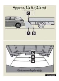
The distance that appears on the screen between three-dimensional objects (such as vehicles) and flat surfaces (such as the road) and the actual distance differ as follows.
