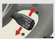
To change the set speed, operate the lever until the desired set speed is obtained.
