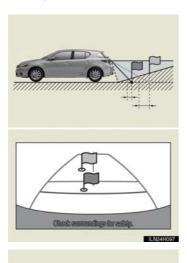
When the grade behind the vehicle slopes up sharply, objects appear to be farther away than they actually are.
