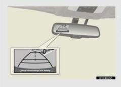
The rear view image is displayed when the shift position is in R and the "POWER" switch is in ON mode.
