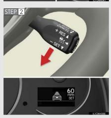
Accelerate or decelerate the vehicle to the desired speed, and push the lever down to set the speed.
