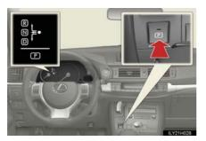
Fully stop the vehicle and set the parking brake, and then press the P position switch.
