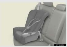
Seat belts equipped with a child restraint locking mechanism (ALR/ELR belts except driver's seat belt) (→P. 86)
