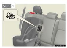
Secure the child restraint system using the seat belt or the LATCH anchors, press the lock release button, and raise the head restraint.
