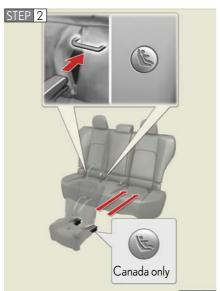
Latch the buckles onto the LATCH anchors. If the child restraint has a top tether strap, the top tether strap should be latched onto the top tether strap anchor.
