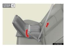
While pushing the child restraint system down into the rear seat, allow the shoulder belt to retract until the child restraint system is securely in place.
