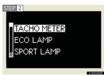
Press the "DISP" switch and select the item, and then press and hold the "DISP" switch.
