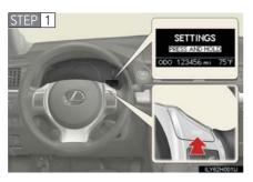
Press the "DISP" switch to display the SETTING screen while the vehicle is stopped, and then press and hold the "DISP" switch to display the customize mode screen.
