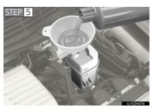
Add power control unit coolant if necessary.
