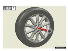
Vehicles with a 16 or 17 inch wheel: Before stowing the flat tire, remove the center wheel ornament by pushing from the reverse side.
