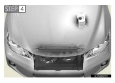
After the hybrid system has cooled down, check the power control unit coolant level and inspect the cooling system for leaks.
