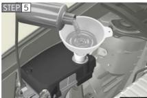
Add engine coolant if necessary.
