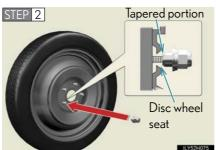
Install the spare tire and loosely tighten each wheel nut by hand by approximately the same amount.
