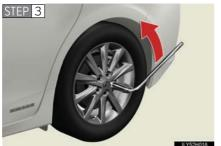
Slightly loosen the wheel nuts (one turn).
