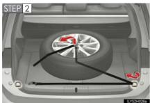
Place the flat tire on the deck board, and pass the belt through the lower-right cargo hook and then through the hole in the center of the tire.
