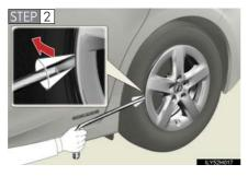
For vehicles with 15 inch wheels, remove the wheel ornament using the wrench.
