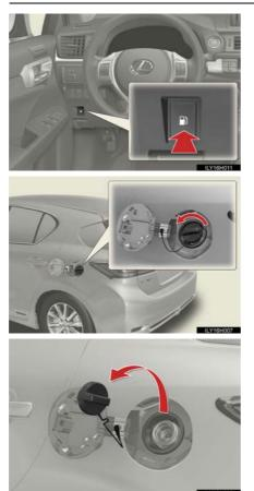
1 Press the opener to open the fuel filler door.
