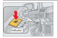
Press the switch down to lock the passenger window.
