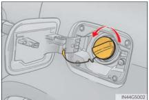
1 With the doors unlocked, press the center of the rear edge of the fuel filler door.
