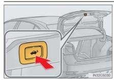
Pressing the switch closes the trunk lid automatically. (A buzzer sounds.)
