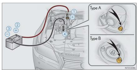
(1) Connect a positive jumper cable clamp to the positive (+) battery terminal on your vehicle.
