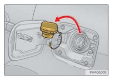
Remove the cover inside the trunk and pull the lever to open the fuel filler door if the fuel filler door cannot be opened pressing the rearward of the fuel filler door.
