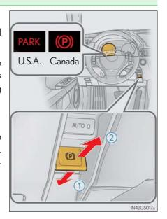
The parking brake is set or released automatically according to shift lever operation.
