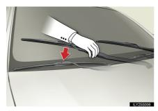
Lower the wipers by pressing on the wiper arm.
