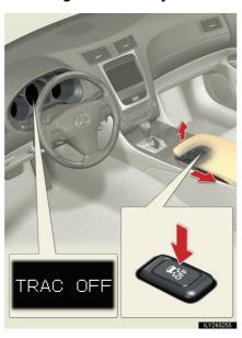
Quickly push and release the button to turn off TRAC.
