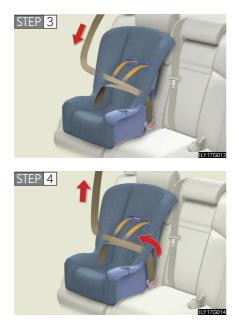
Fully extend the shoulder strap and then allow it to retract slightly into the ALR lock mode.
