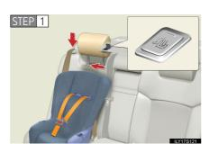
Secure the child restraint system using a seat belt or lower anchors, and move the head restraint in place at the lowest position.
