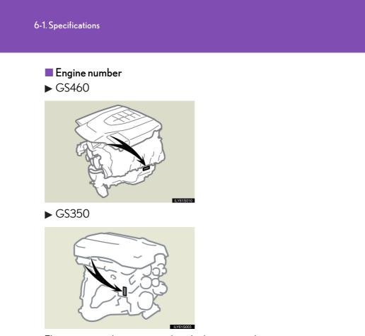
The engine number is stamped on the location as shown.
