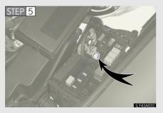
Remove the fuse with the pullout tool.
