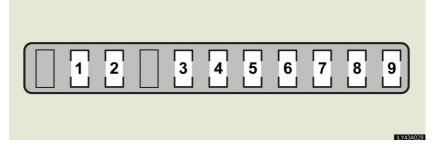
Fuse Ampere Circuit RR S/SHADE 7.5 Rear sunshade PSB 30 2 Pre-collision seat belt 3 RR-IG2 10 Pre-collision seat belt, seat belt pre-4 RR-IG1 10 tensioners, A/P UNIT, rear sunshade RR-B 5 10 Trunk light, noise filter **RR FOG** 7.5 6 STOPLPL 7 10 Stoplights, back-up light 8 STOP LP R 10 High mounted stoplights Tail lights, license plate lights, rear 9 **RR TAIL** 10 side marker lights
