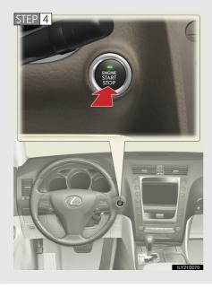
Press the "ENGINE START STOP" switch.
