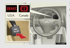
Sets the parking brake<sup>\*</sup> (Depressing the pedal again releases the parking brake.)
