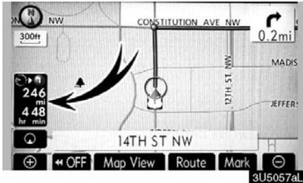
When the vehicle is on the guidance route, the distance and the estimated travel/arrival time to the destination are displayed. When the vehicle is not on the guidance route, the distance and the direction of the destination are displayed.
