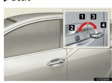
Using the mechanical key  $(\rightarrow P.25)$ in order to perform the following operations:
