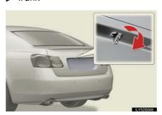
Turn the mechanical key clockwise to open.
