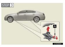
Turn the tire jack portion "A" by hand until the notch of the jack is in contact with the jack point.
