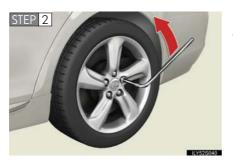
Slightly loosen the wheel nuts (one turn).
