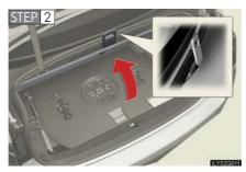
Secure the panel using the hook provided. Then take out the tool tray.
