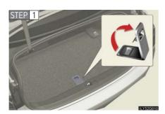
Lift up the hook of the panel on the trunk floor.
