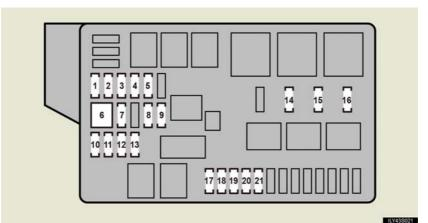
Fuse Circuit Ampere H-LP UPR and HORN FR CTRL-B 25 1 A/F 2 15 Exhaust system 3 ETCS 10 Electronic throttle control system 4 ALT-S 7.5 Charging system Multiport fuel injection system/ INJ2 25 5 sequential multiport fuel injection system H-LP CLN 6 30 Headlight cleaner STB-AM 7 30 25 8 DEICER 9 FR CTRL-AM 30 FR TAIL, FR FOG and WASHER
