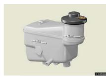
The brake fluid level should be between the "MAX" and "MIN" lines on the tank.
