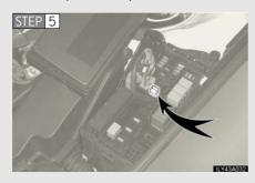
Remove the fuse with the pullout tool.
