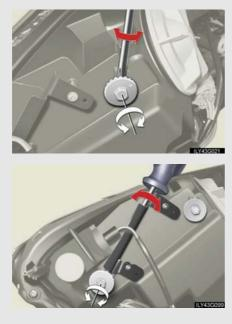
Using a Phillips-head screwdriver, turn adjustment bolt A so that the bubble is within the 2 center lines.
