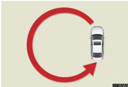
If "CAL" appears on the display, drive the vehicle at 5 mph (8 km/h) or less in a circle until a direction is displayed.
