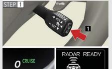
1 Press the "ON-OFF" button to activate the cruise control.
