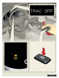
Push and hold the button for more than 3 seconds while the vehicle is stopped to turn off TRAC and Enhanced VSC.
