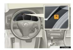
If the vehicle is in danger of slipping, rolling backwards when starting on an incline, or if the rear wheels (2WD models) or all wheels (4WD models) spin, the slip indicator light flashes to indicate that the Enhanced VSC/TRAC/hill-start assist control systems have been engaged.
