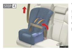
While pushing the child restraint system into the rear seat, allow the shoulder belt to retract until the child restraint system is securely in place.
