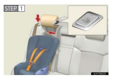
Secure the child restraint system using a seat belt or lower anchors, and move the head restraint in place at the lowest position.
