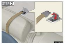
Open the anchor bracket cover, latch the hook onto the anchor bracket and tighten the top tether strap.
