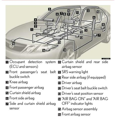
Your vehicle is equipped with "ADVANCED AIRBAGS" designed based on US motor vehicle safety standards (FMVSS208). The airbag system controls airbag deployment power for the driver and front passenger. The driver airbag system consists of the driver's seat position sensor etc. The front passenger's airbag system consists of the front passenger occupant classification sensor etc.
