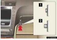
To disable the trunk opener, turn OFF the main switch in the glove box.
