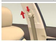
To raise: pull the anchor upward.
