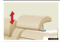
Height adjustment: to raise the head restraint, pull it upward. To lower the head restraint, push it down while pressing the lock release button.
