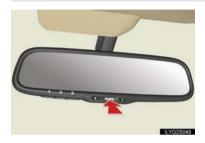
To turn auto mode on/off, press the auto button. The indicator comes on when auto mode is turned on.
