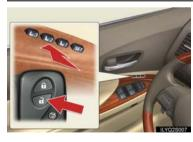
While holding the desired memory button, press and hold abutton on the wireless remote control until you hear a beep.
