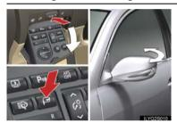
To fold the mirrors, press the button. Press the button again to return them to the extended position.
