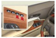
While holding the "SET" button, press and hold one of the memory buttons ("1", "2", or "3") until you hear a beep.
