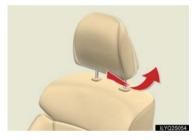
Grip the head restraint and twist to tilt forward or backward.
