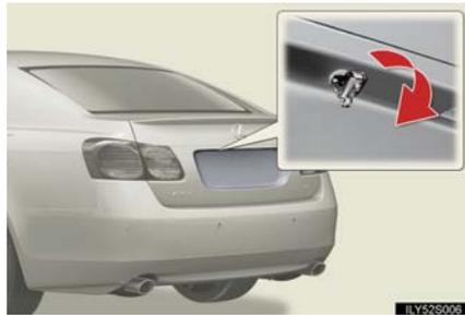
Turn the mechanical key clockwise to open.
