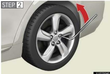
Slightly loosen the wheel nuts (one turn).
