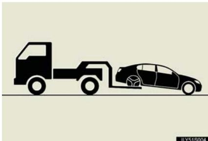
Turn the "ENGINE START STOP" switch to the ACCESSORY mode so that the steering wheel is unlocked.
