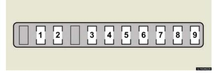
Ampere Circuit RR S/SHADE 7.5 Rear sunshade 2 PSB 30 Pre-collision seat belt 3 RR-IG2 10 Pre-collision seat belt, seat belt pre-RR-IG1 10 4 tensioners, A/P UNIT, rear sunshade 5 RR-B 10 Trunk light, noise filter **RR FOG** 7.5 7 STOPLPL 10 Stoplights, back-up light STOP LP R 8 10 High mounted stoplights Tail lights, license plate lights, rear 9 **RR TAIL** 10 side marker lights
