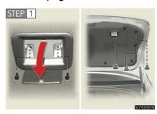
Open the trunk lid. Remove the trunk handle and panel cover clips.
