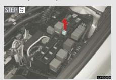
Remove the fuse with the pullout tool.
