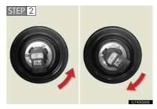
Turn the bulb base counterclockwise to remove it.
