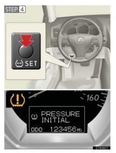
Push and hold the tire pressure warning reset switch until the tire pressure warning light blinks slowly three times and the message "PRESSURE INITIAL" appears on the multi-information display.
