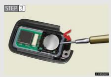
Remove the depleted battery.
